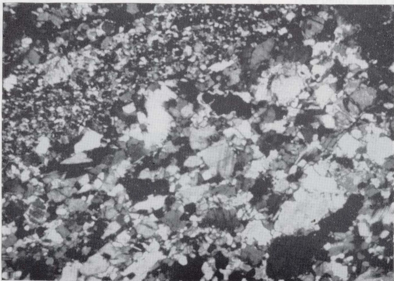
Fig. 9.—Photomicrograph showing a significant grain-size reduction that typically occurs at the chilled margin of the dikes shown on fig. 8.
